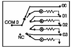
Model 1260-54 consists of six of the above 1x4 tree multiplexers. Each channel has the capability of being terminated to an optional  $50\Omega$  terminator. One tree is shown.
